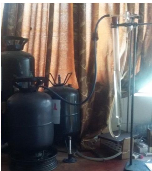
PLATE 3.1f: Experimental setup (digester and gasometric chamber)
