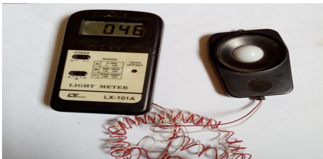
Plate 1: LX 101A Light Meter Used in the Collection of Data From the Field
