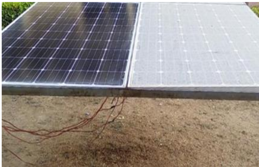
Figure 2: Experimental Setup for Effects of Dust on PV module
