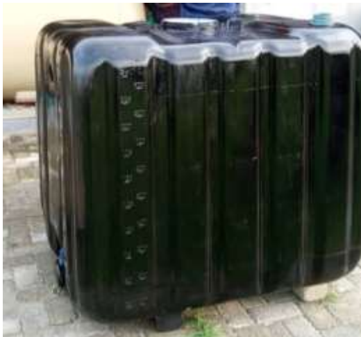
Figure 5: Biodigester Liner Coated with Black Paint
