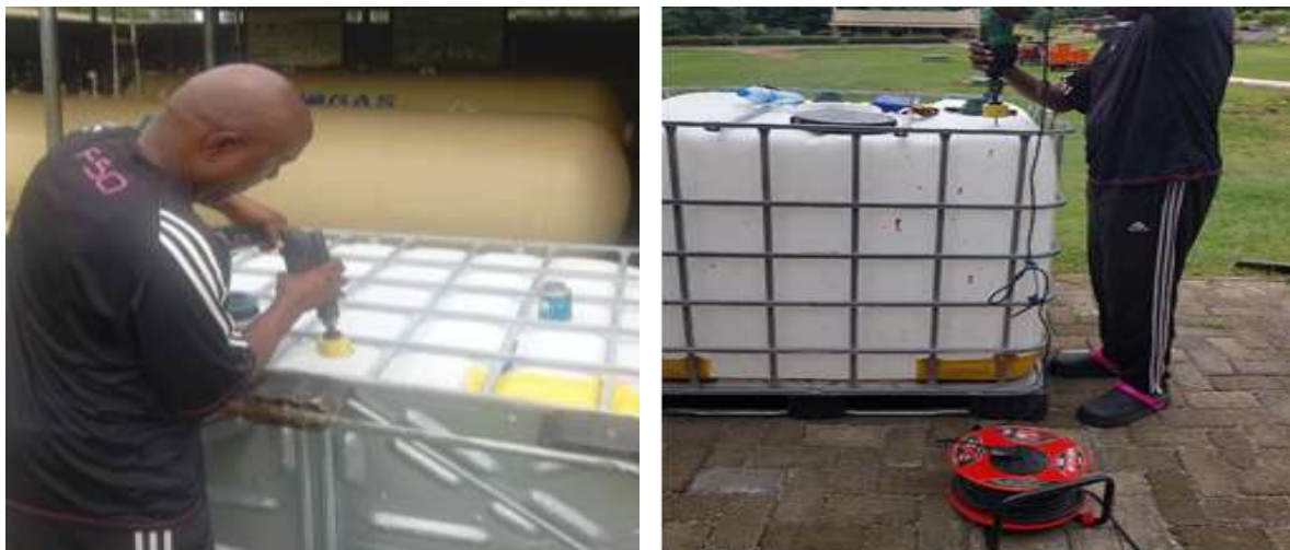
Figure 7: Drilling Process of the 1000 Litres Capacity IBC Tank
