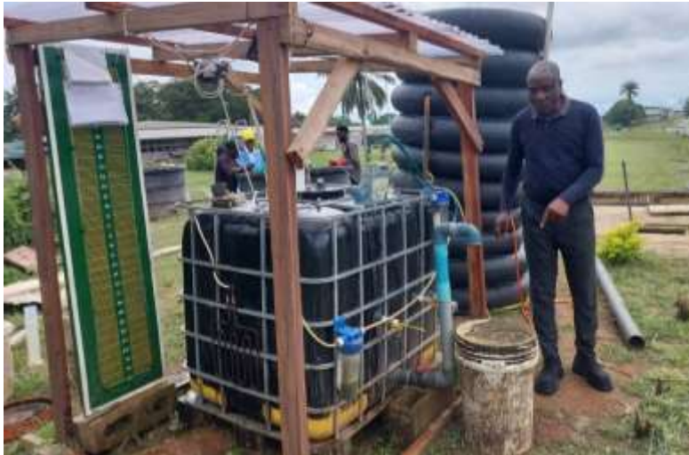
Figure 9: Biofertilizer effluent from Bottom outlet and Biogas collection in Tyre tubes
