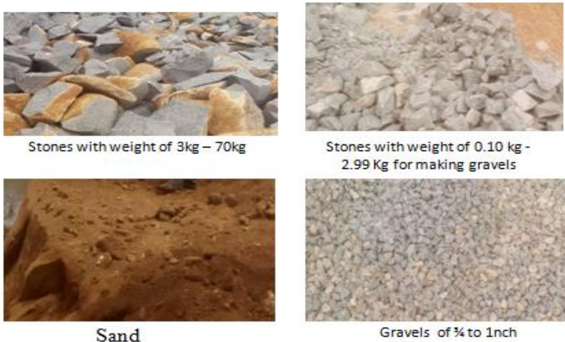
Plate 1: Types of building material extracted traditionally in mining sites
