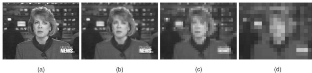
. (a) n = 1 , original image. (b) n = 4 . (c) n = 8 . (d) n = 16 . Original and corresponding low resolution images. Each square cell consists of pixels in which the intensity of each pixel is replaced by the average intensity of the pixels in that cell.
