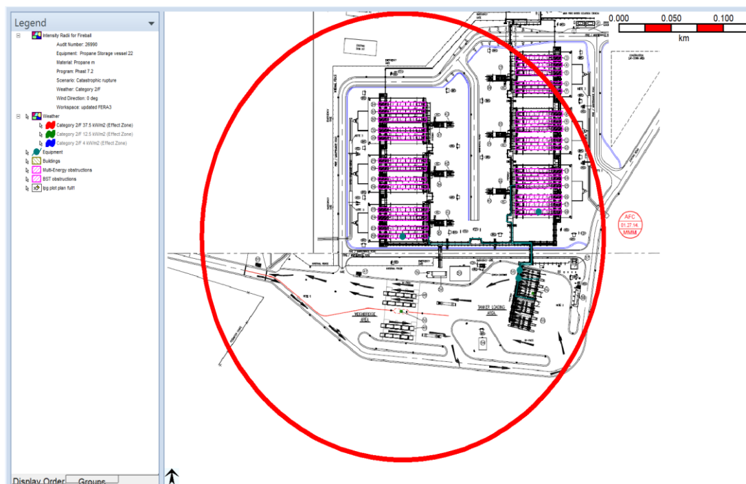
Fig 17: Impacted Zone of Thermal Radiation Intensity of 37.5 KW/m 2 due to Fireball from Catastrophic Failure of the Propane Pressure Vessel #22 at 2/F Weather Category
