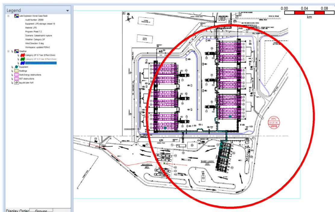
Fig 18: Impacted Zone of Explosion Overpressure Contour of 0.7bar due to Catastrophic Rupture case of LPG vessel #18 at 2/F Weather Category
