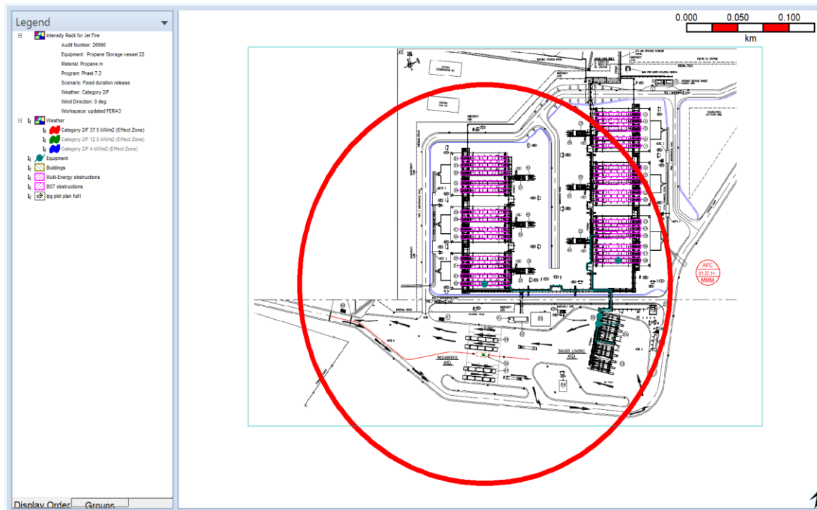
Fig 16: Impacted Zone of Thermal Radiation Intensity of 37.5 kW/m 2 due to Jet Fire from Fixed Duration Release of Propane Vessel #22 at 2/F Weather Category
