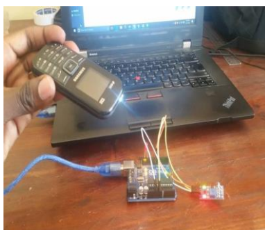
Figures 29 and 30: Showing the Photosensitive Sensor Module Connection – Day Light ON, Photosensitive Sensor Module Connection – Day Light OFF respectively.
