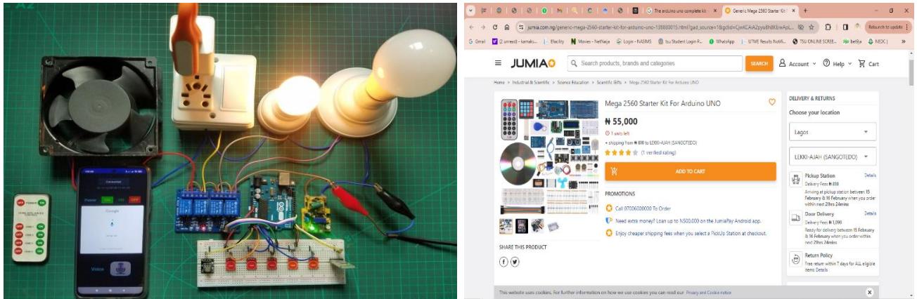
Figures 35 and 36: Arduino UNO integrated with Android (Control), Relays, Loads (Switches), Fans, Bluetooth HC-06, MQ-2 and Photosensitive Sensor & Arduino UNO M-2560 Starter Kit Price (Jumia, 2024)
