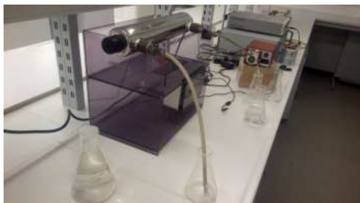
Figure 1. UV irradiation chamber.
