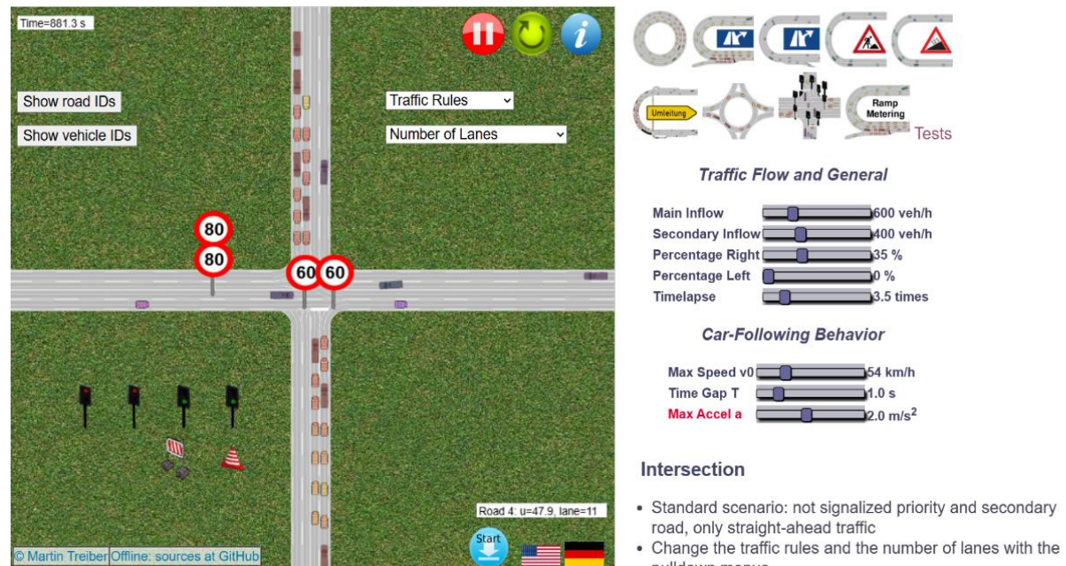
Figure 2: Simulation of Traffic Flow Impact Due to Lane Changing Behavior
