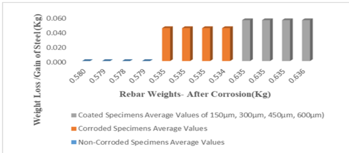
Figure 17: Average Rebar Weights- After Corrosion (Kg) versus Weight Loss /Gain of Steel (Kg)
