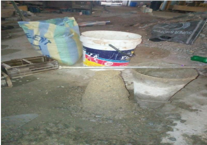
Figure 2: The slump of concrete made by replacing river sand with sawdust at 10%
