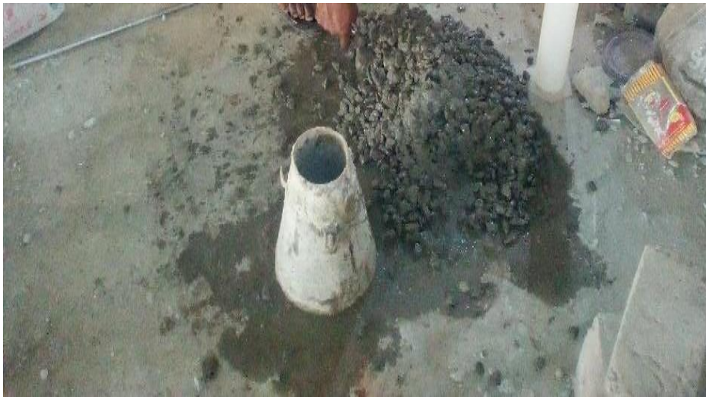
Figure 1: Concrete Hand Mixing in the Laboratory
