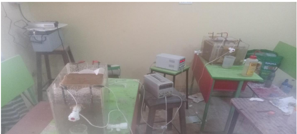
Figure 1: Laboratory set-up for the Electrokinetic Remediation Process
