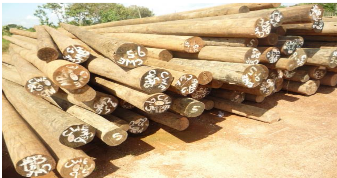
Fig 3.2 Some finished CCA treated poles packed in the sun ready to be transported across the nation.
