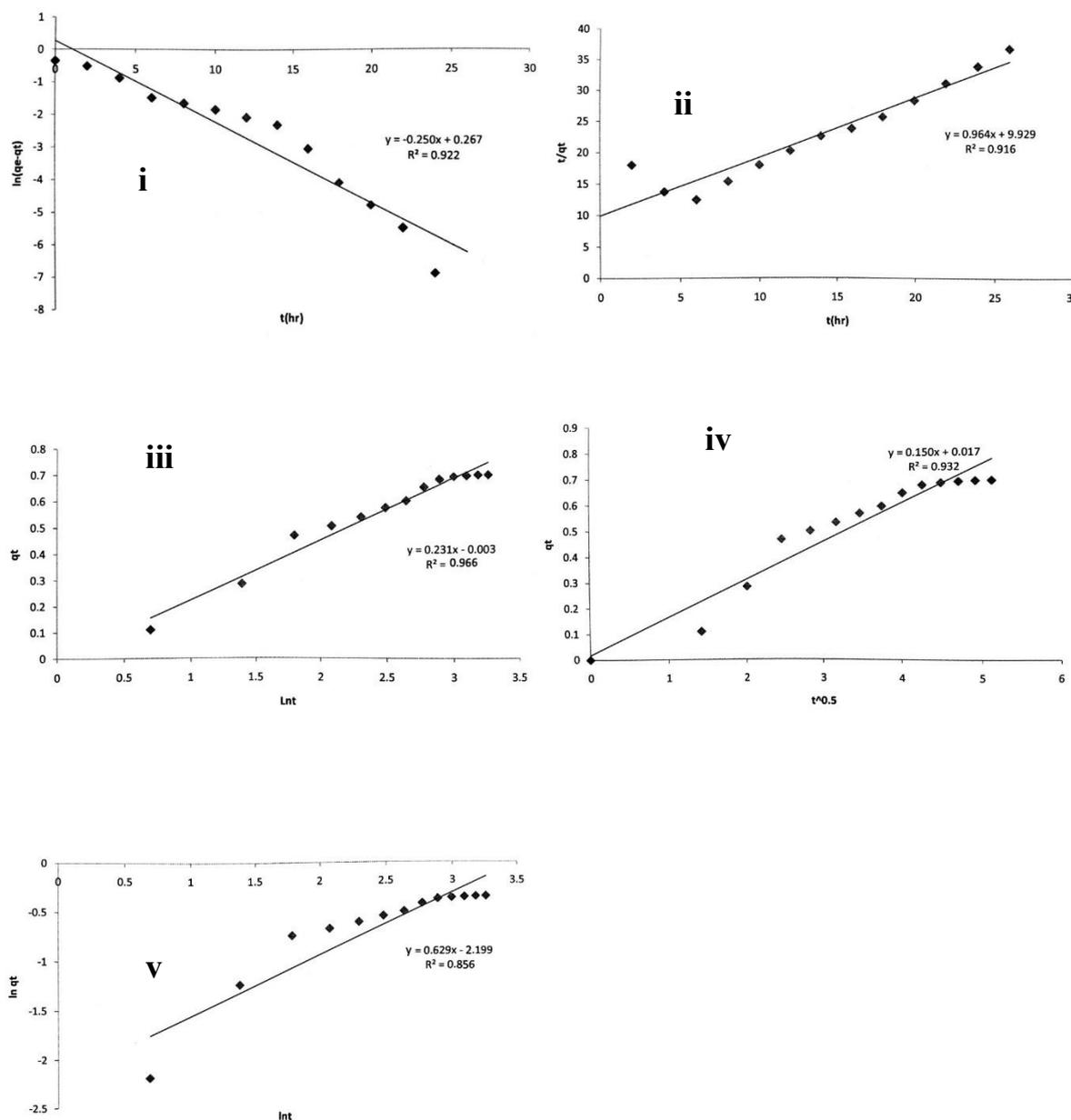
Figure 5: Models' Output for Adsorption of Benzene on modified Clay
