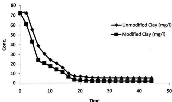
**Figure 2 - Equilibrium Time for Adsorption of Benzene on unmodified and calcined Modified Clay.**
