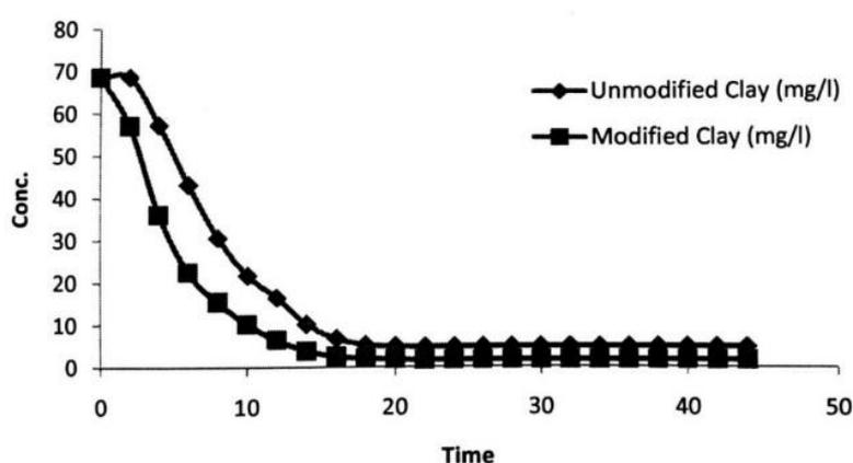
**Figure 3. - Equilibrium Time for Adsorption of Naphthalene on unmodified and calcined modified clay**
