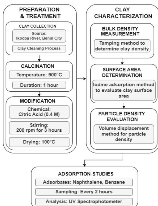
**Figure 1: Adsorption of Naphthalene and Benzene Architecture**
