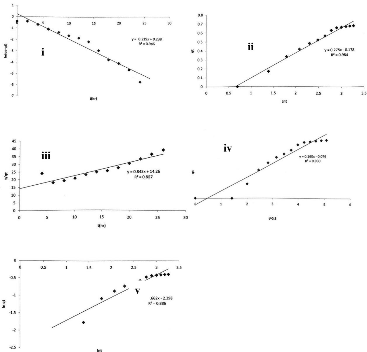
**Figure 4: Models' outputs for Adsorption of Benzene on Unmodified Clay**
